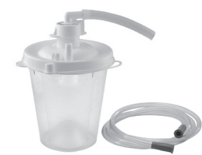
Assembled Collection Container Kit 7305D-633 - Includes 800 ml container and lid, internal filter cartridge, splash guard, and 4.5" (11.43 cm) connection and 6' (1.8 m) patient tubing (1/ea)
